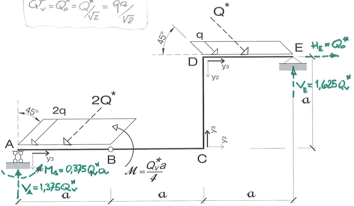
$$\left. \begin{aligned} \sum F_o = 0 &\Rightarrow -2Q_o^* + Q_o^* - H_E = 0 \Rightarrow H_E = Q_o^* \\ \sum M_B^{dx} = 0 &\Rightarrow V_E 2a - H_E a - Q_o^* a - Q_v^* \frac{3a}{2} + Q_v^* \frac{a}{4} = 0 \\ &V_E = 1,625 Q_v^* \\ \sum F_v = 0 &\Rightarrow -V_A + 2Q_v^* + Q_v^* - V_E = 0 \Rightarrow V_A = 1,375 Q_v^* \\ \sum M_B^{sx} = 0 &\Rightarrow -V_A a + 2Q_v^* \frac{a}{2} + M_A = 0 \Rightarrow M_A = 0,375 Q_v^* a \end{aligned} \right\}$$
